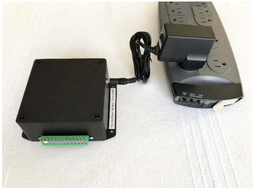
**Step 3:** Using a small screwdriver, attach the connector wire to the controller box. Match the wire colors with the sticker colors on the controller box. The diagram in the top left corner of the picture is a close up of the wires attached to the controller box. Tighten firmly so a gentle tug test will not pull the wire out of the controller box but there is no need to over do it. Climbers do tend to have strong hands!
