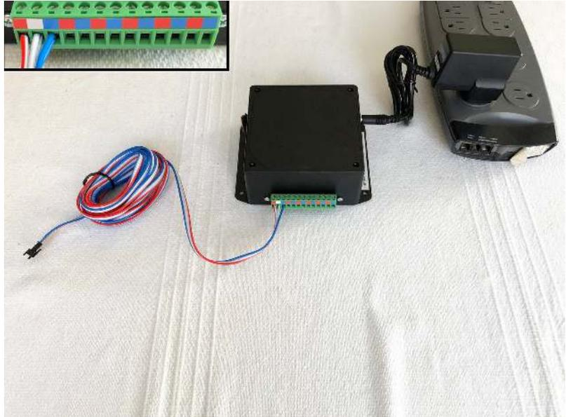
**Step 4:** Attach the input end of the first LED string to the connector wire. Attach the power injection wires at the output end of the first LED string to the controller box. Ensure all wire and sticker colors match.
