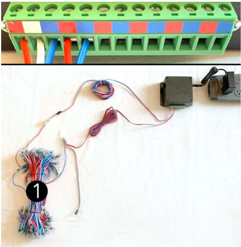
**Step 5:** Attach the input end of the second LED string to the output end of the first LED string. Attach the power injection wires at the output end of the second LED string to the controller box.
