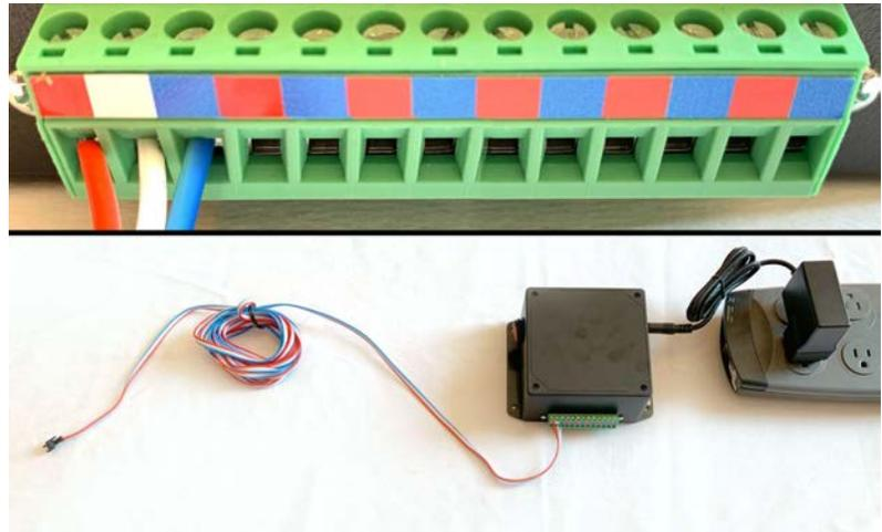
**Step 4:** Attach the input end of the first LED string to the connector wire. Attach the power injection wires at the output end of the first LED string to the controller box. Ensure all wire and sticker colors match.
