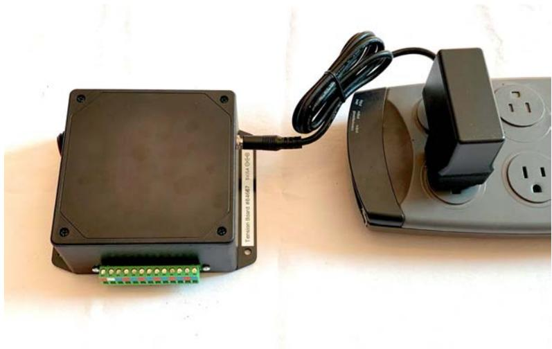
**Step 3:** Using a small screwdriver, attach the connector wire to the controller box. Match the wire colors with the sticker colors on the controller box. The diagram in the top of the picture is a close up of the wires attached to the controller box. Tighten firmly so a gentle tug test will not pull the wire out of the controller box but there is no need to over do it. Climbers do tend to have strong hands!
