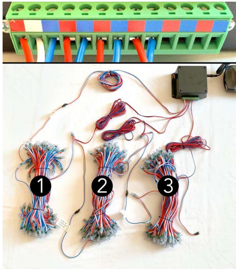
**Step 7:** Attach the input end of the fourth LED string to the output end of the third LED string. Attach the power injection wires at the output end of the fourth LED string to the controller box.
