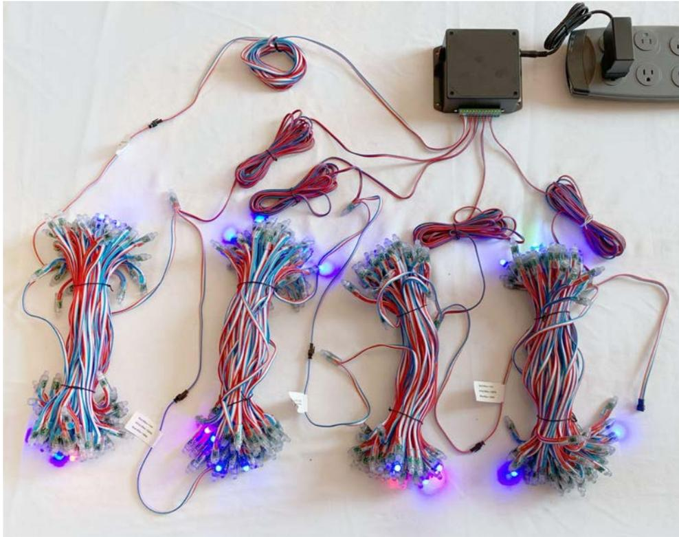
**Step 9:** Disconnect all the pieces of the LED kit in preparation for installing the LED kit on your Tension Board 2.
